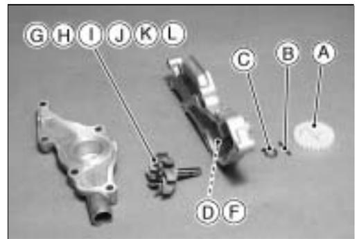
**Internal Parts — Mechanical Seal**
