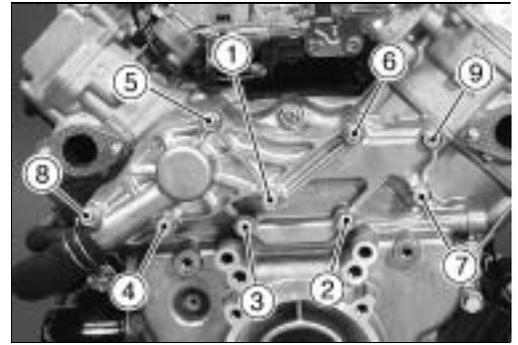
**Water Pump Disassembly**
