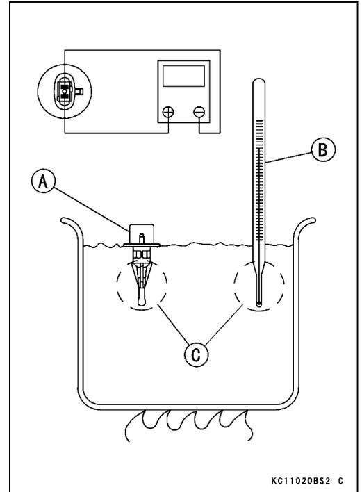
Water Temperature Sensor (Fault Code 13)
