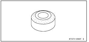
Valve Seat Cutter, 32° -  $\phi$ 35: 57001-1121
