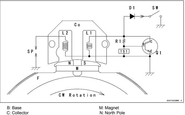
C: CollectorN: North PoleCo: Core (Lamination)R1: Control ResistorD1: DiodeS: South PoleE: EmitterSP: Spark PlugF: FlywheelSW: Stop SwitchL1: Primary CoilTS1: Trigger SensorL2: Secondary CoilQ1: Transistor
