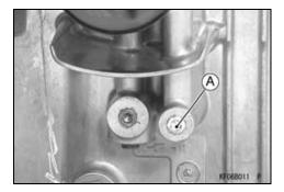
• Install the oil pressure gauge adapter [A] and oil pressure gauge [B].
