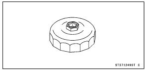
Valve Seat Cutter Holder,  $\phi$ 6: 57001-1360
