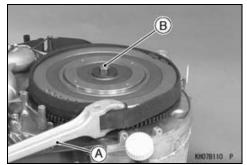
• Remove: Bolts [A] Fan Housing [B]
